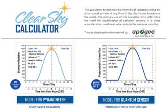
Homepage of the Clear Sky Calculator. Two calculators are available: one for quantum sensors (PPFD) and one for pyranometers (total shortwave radiation).
